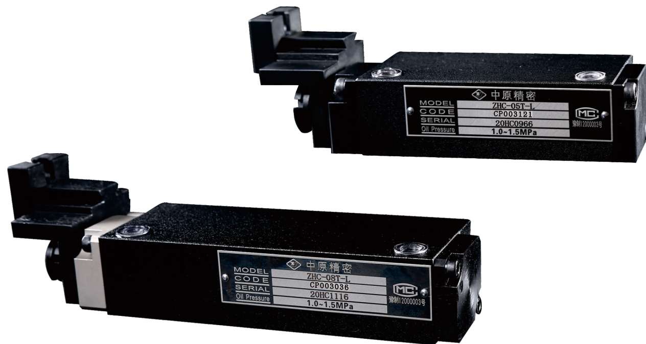
The external view of OD gaging unit and horizontal hydro-cylinder
